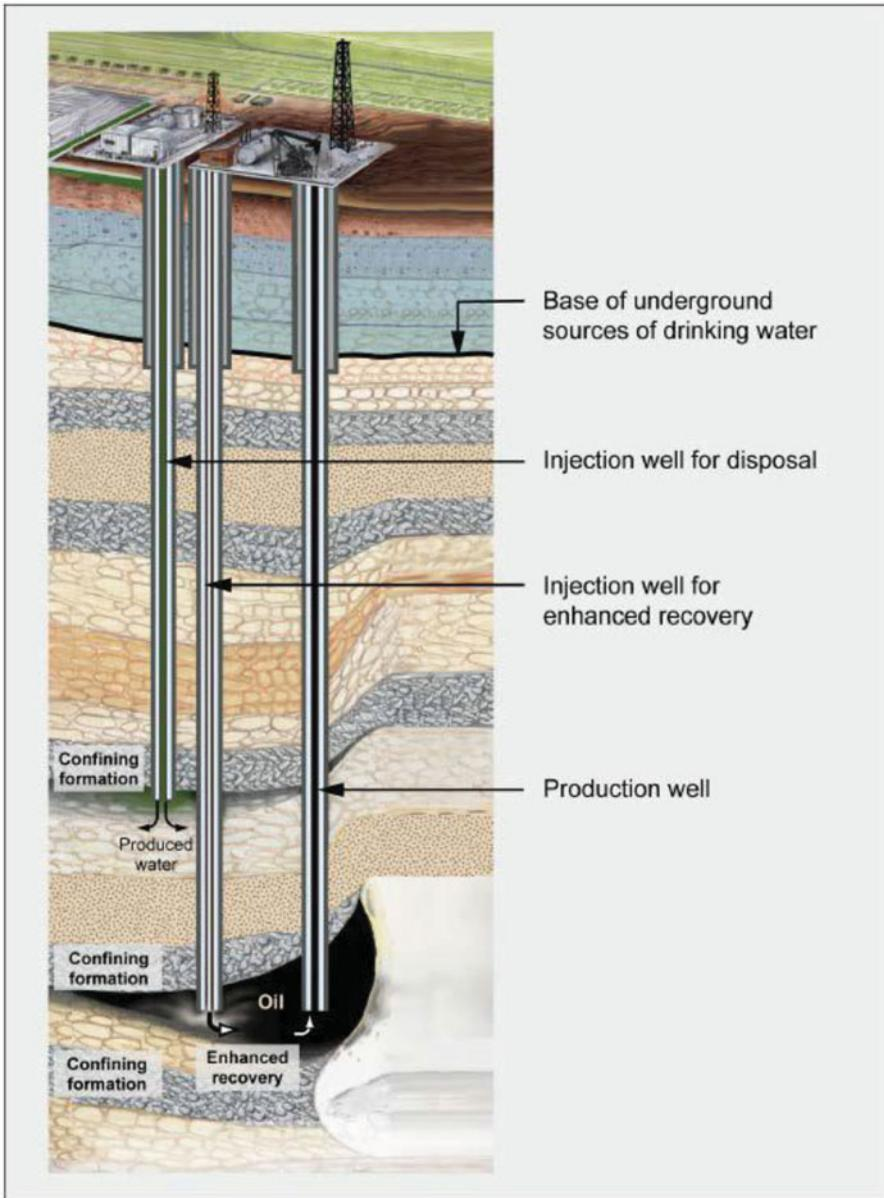
**Figure 2.** Injection wells for enhanced production and wastewater disposal.
